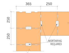
- CORNER BONDING, 1ST ROW OF BRICKWORK
