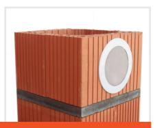
3. If the combustion air supply adapter is used, cut a 170 mm diameter round hole in the centre of the chimney wall at the required height. Glue the stainless steel transition adapter into the hole using adhesive mortar (HLM). Cut a hole in the rubber membrane according to the diameter of the pipe to be connected. To ensure tightness, the opening in the membrane must always be smaller than the diameter of the pipe to be connected.
